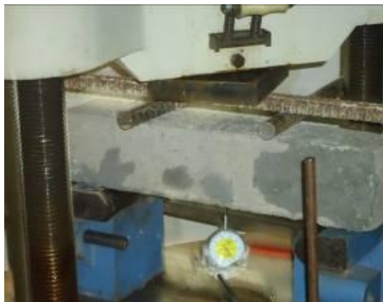
PLATE 3: Experimental Set Up and Progress Photograph of Flexural Test
