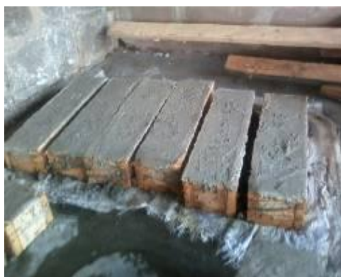
PLATE 2: Beam Specimens during casting and during wet curing
