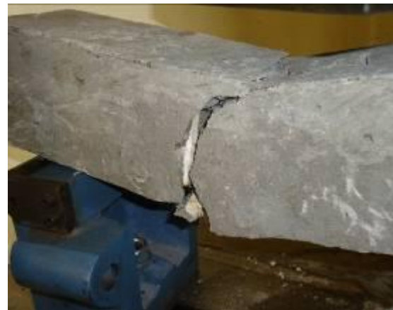
PLATE 4: Failure mechanism and crack pattern in typical experimental beam.
