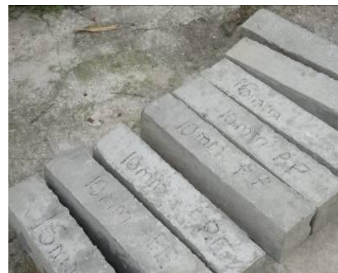
PLATE 2: Beam Specimens during casting and during wet curing
