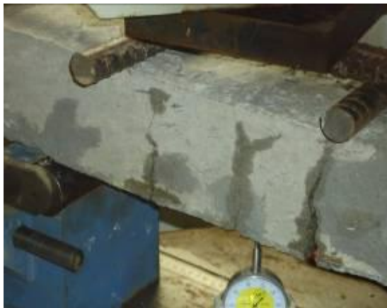
PLATE 4: Failure mechanism and crack pattern in typical experimental beam.
