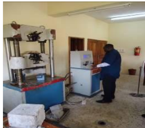
PLATE 3: Experimental Set Up and Progress Photograph of Flexural Test
